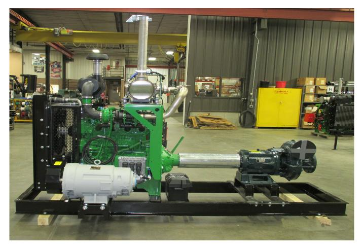
John Deere **4045 Final Tier 4** skid mounted pumping unit and generator. With Cornell frame mounted pump shown.
