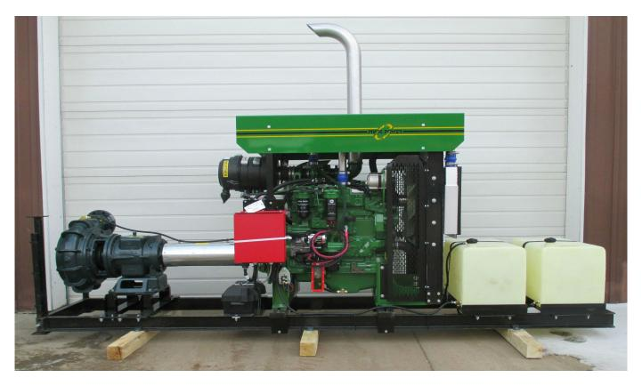
John Deere 4045 trailer mounted pumping unit with Cornell frame mounted pump. Shown with optional fuel tanks.
